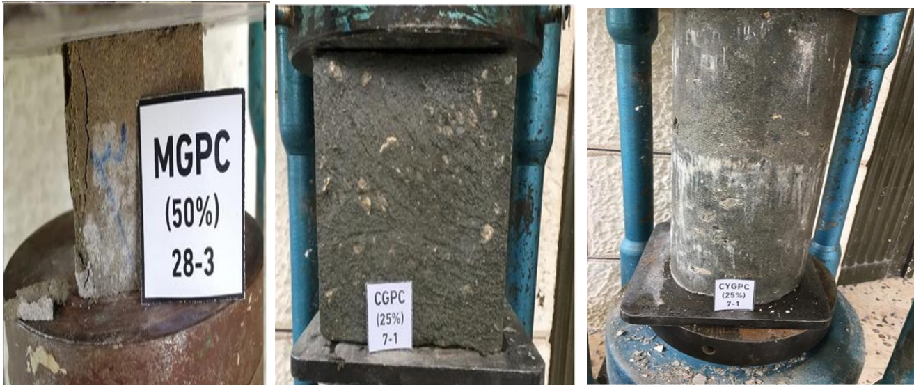
Figure.2: Resistance strength experiments for (A) Masonry cubes with 50%Phosphorite wastes and 50%Gypsum, (B) Phosphorite wastes fine and Gypsum concrete cubes, (C) Phosphorite wastes fine Gypsum concrete cylinders.
