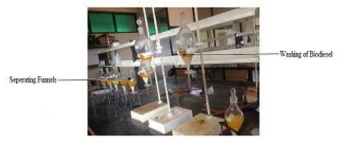
Fig. 3. Washing and distillation process
