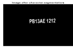
Fig. 12. Image obtained after character segmentation
