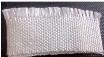
Figure 5. Two-Directional glass fiber sheets
