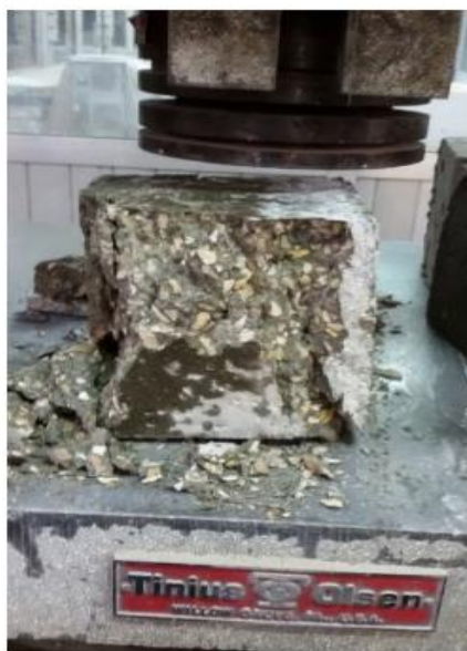
Figure 3. Control Specimen after Compression test.
