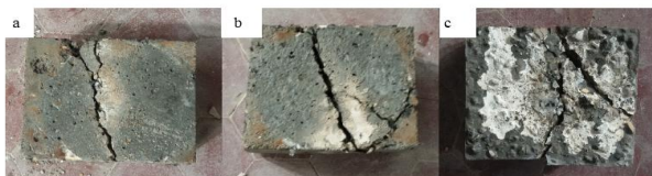
Figure 11. Impact test (a) C-10, (b) C-20, (c) C-30.
