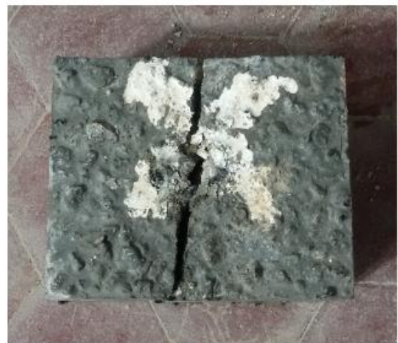
Figure 9. Control Specimen after impact test.
