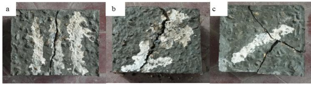
Figure 10. Impact test (a) F-10, (b) F-20, (c) F-30.
