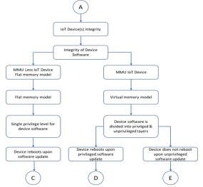
Fig. 3. Classifying IoT devices based upon their memory model & behavior on software update
