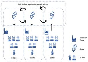
Fig. 2. IoT devices network topology in typical large factory environment
