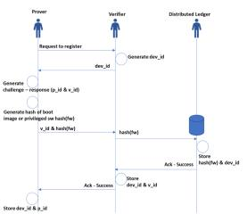
Fig. 5. Registering device boot attestation parameters during initialization or software update
