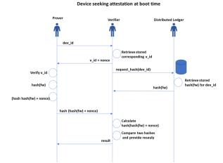
Fig. 6. Device seeking attestation at boot time
