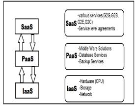
Fig.2.1 – The models of cloud computing
