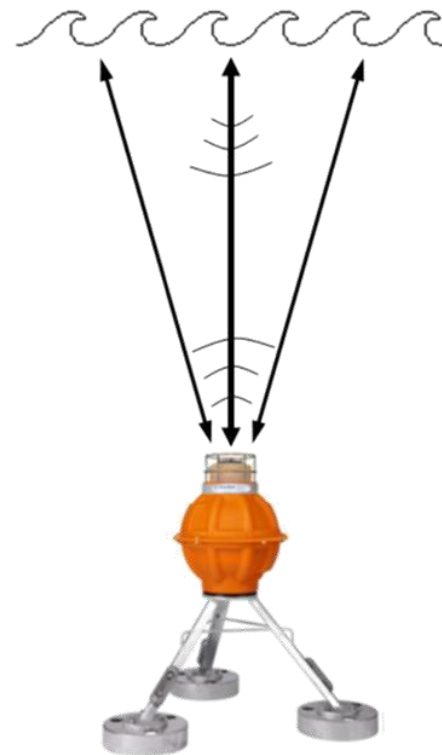
A Pressure Inverted Echo Sounder (Wang et al. , 2012).
