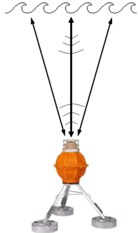
A Pressure Inverted Echo Sounder (Wang et al. , 2012).
