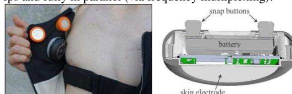
Figure 1: Wearable EIT belt integrated in a vest (left) and example of integration of a CS (right) with a diameter of 38 mm.
