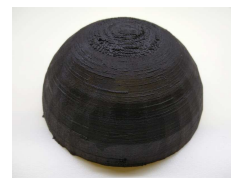
Figure 2: Simple hemispherical anatomically accurate breast phantom created using heterogeneous mixture of the two tissues.
