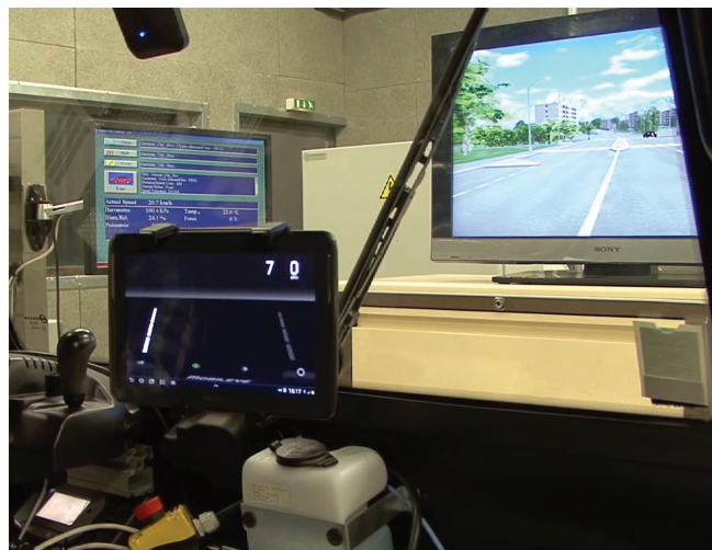
Figure 11.10 Lane departure warning triggered.
