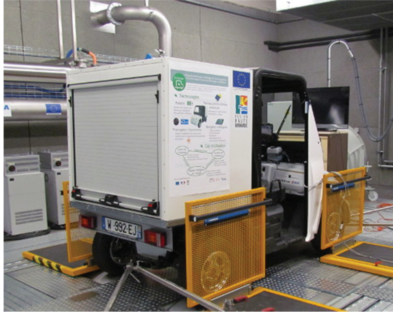
Figure 11.7 The Biocar test vehicle on the Horiba chassis dynamometer.
