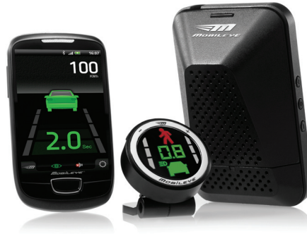
Figure 11.5 Mobileye 560 aftermarket vision-based ADAS.
