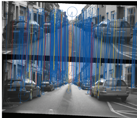
Figure 8.21 Comparison of the resulting pixel correspondences for the 8 bpp and 12 bpp input images. In the 12 bpp input image, an overall number of 611 pixel pairs has been detected, whereas in the 8 bpp input image 608 correspondences have been determined. A subset of 587 pairs (96.1%) is identical in both images (blue lines). Furthermore, there are 23 (3.8%) exclusive 8 bpp pairs (red lines) and 24 (3.9%) exclusive 12 bpp pixel correspondences (orange lines).
