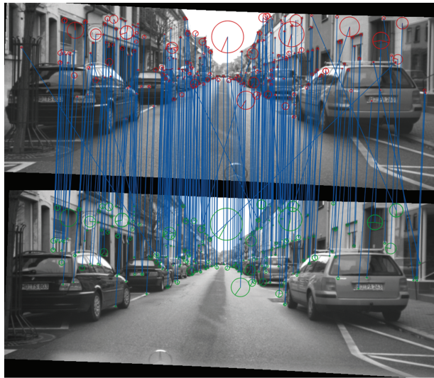
Figure 8.2 Left ( top ) and right ( bottom ) image from a stereo camera system showing detected SIFT-image features. Detected feature points of the left/right image are displayed in red/green, matches are displayed in blue. Scale and rotation of the SIFT-features are illustrated by the circle properties.
