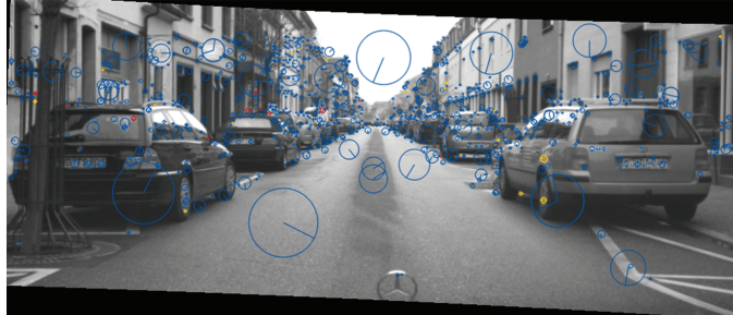
Figure 8.20 Comparison of the resulting SIFT-features of the left input image for 12 bpp images and 8 bpp images. In the 12 bpp input image, an overall number of 1,069 features have been detected, whereas in the 8 bpp input image 1,056 features have been determined. A subset of 1,045 features (97.8%) is identical in both images (blue). There are 14 (1.3%) exclusive 8 bpp feature positions (red) detected and 24 (2.2%) exclusive 12 bpp feature positions (orange).
