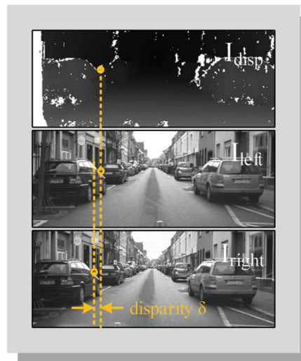
Figure 8.19 Verification of match positions with disparity maps. For rectified images, the horizontal difference of feature positions of a corresponding pixel pair equals the related value of the disparity map. With this technique, it is possible to validate resulting matching lists for datasets with ground truth disparity maps.
