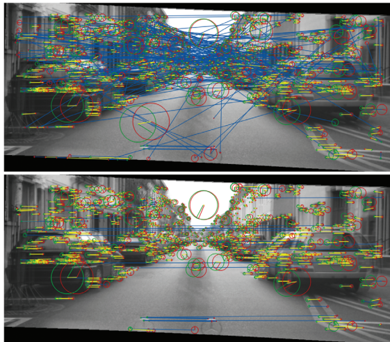
Figure 8.18 Exemplary results of feature matching. The left and right stereo images are overlaid; features of the left/right image are displayed in red/green. Correct matches are depicted in yellow; false matches are shown in blue. The upper image shows the results of the initial brute force matching, whereas the lower image shows the results of the enhanced matching process.
