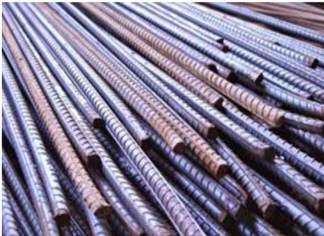
Fig. 1 Y-bar reinforced steel
