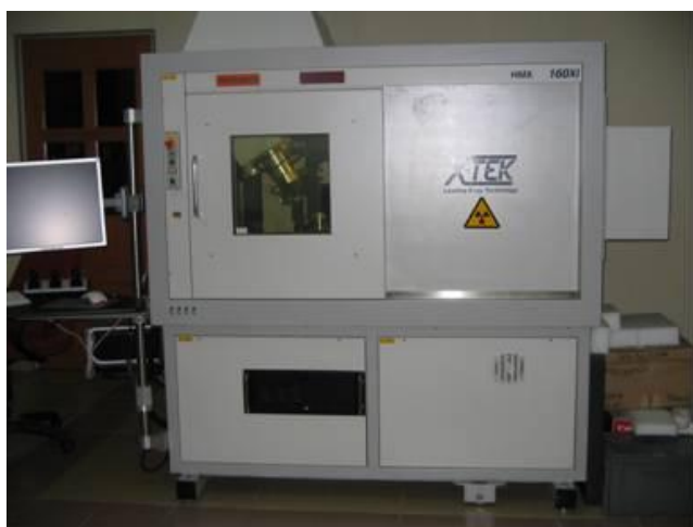
Fig. 2 Non-destructive technique using X-ray imaging system model HMX 160Xi
