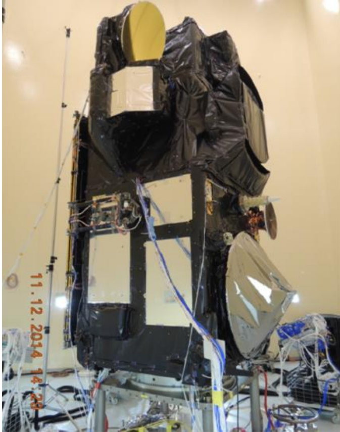
S3A Satellite on stand within the Acoustic Chamber at Thales Alenia Space in Cannes (Courtesy TAS-F)
