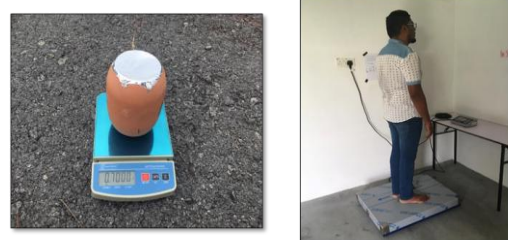
Fig. 2. Measurement of human and porous material by using electric precision balance scale
