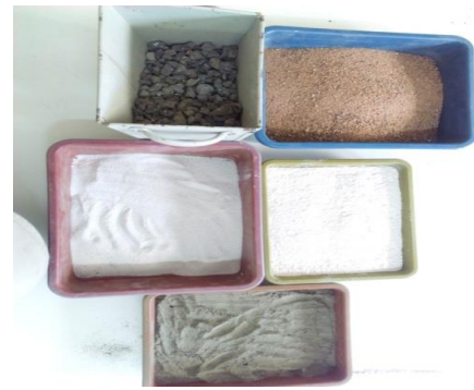
Fig. 1 SCC ingredients for Design mix M30
