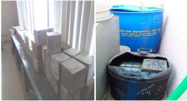
Fig. 2 Acid and sulfate attack test specimen arrangement
