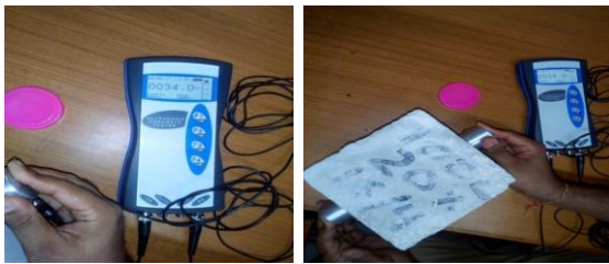
Fig.8 Ultrasonic pulse velocity test
