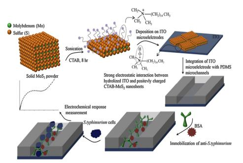
**Figure 11.** Design of a MoS<sub>2</sub> based biosensor for *S. typhimurium* detection. Adapted with permission from [145] Copyright 2018, Elsevier.
