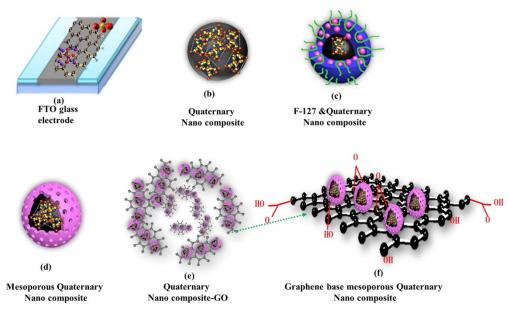
**Figure 3.** Schematic presentation of the synthesis process of the ZrO<sub>2</sub>-Ag-Graphene Oxide -SiO<sub>2</sub> nanocomposite. Adapted with permission from [46] Copyright 2020, American Chemical Society.
