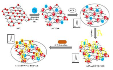
**Figure 4.** Schematic presentation of the fabrication of rGO-TiO<sub>2</sub> electrodes and their employing for electrochemical detection of bacteria. Adapted with permission from [60] Copyright 2019, Elsevier.
