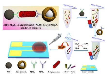
**Figure 5.** Illustration of the detection of *S. typhimirium* using immunomagnetic separation and impedance monitoring of the release of Mn<sup>2+</sup> from the SiO<sub>2</sub>@MnO<sub>2</sub> nanocomposite. Adapted with permission from [65] Copyright 2020, Elsevier.
