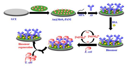
**Figure 9.** Schematic representation of the label-free electrochemical biosensor based on Au@MoS<sub>2</sub>– PANI. Adapted with permission from [128] Copyright 2021, MDPI.
