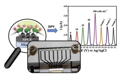
**Figure 10.** The microfluidic device connectors and the eight magnets externally attached with double-sided tape over each working electrode, together with a schematic representation of detection. Adapted with permission from [134] Copyright 2018, Elsevier.
