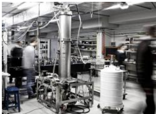
Figure 1.2: IT-CsF2 [2], caesium fountain that constitutes the primary frequency standard for Italy. It is conserved at INRiM in Torino
