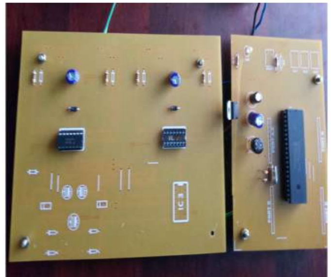
Fig12. Driver circuit interfaced with PIC microcontroller
