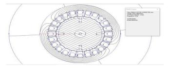
can observe the more number of flux lines cutting the rotor Fig 25. Flux distribution
