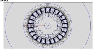
Fig 17.Grey Scale representation of Flux density field 6. Finding the vector direction of Magnetic field
