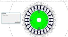
Fig 19. Magnetic field co-energy calculation
