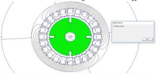
Fig 29. Magnetic field co-energy calculation 8. Calculation of Magnetic field energy This is similar to the magnetic field co energy calculation.
