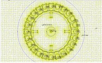
Fig 26. Area selection for characteristics 5. Grey scale representation for flux density distribution The grey scale plot is similar to the density plot it helps in the better understanding of the magnetic flux density
