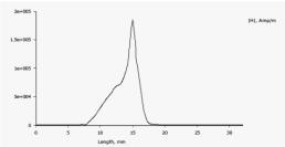
Fig 21. Plot of Magnitude of Magnetic field intensity v/s length of selected lines
