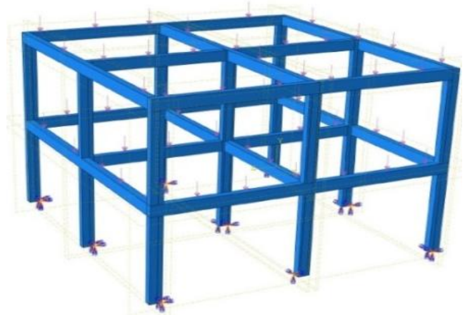
Fig. 3. Assembly and Support condition of Model-1
