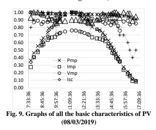
Retrieval Number: D8032049420/2020©BEIESP DOI: 10.35940/ijeat.D8032.049420 Journal Website: <u>www.ijeat.org</u> The table below shows the values of the graphs shown in Figure 9. In the table, the values of the maximum power point, current at the maximum power point, voltage at the maximum power point, short circuit current, and open circuit voltage are shown relative to time.
