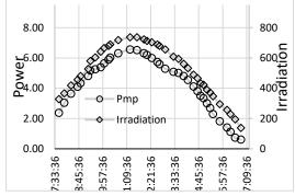
Fig. 8. Change in solar radiation during the day and comparison with the points of maximum power of the PV (08/03/2019, the angle of inclination is 51 ° and the azimuth angle is -34 °).
