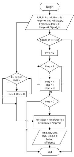
Fig. 4. The block diagram of the software algorithm with the search for the maximum power point.
