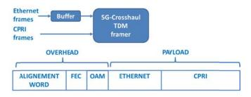
Figure 2: Simple TDM scheme for fronthaul and backhaul multiplexing
