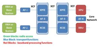
Figure 4: 5G-Crosshaul data plane architecture
