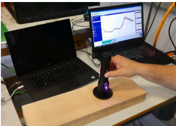
Fig. 2. MicroNIR OnSite-W sensor used for off-line manual acquisition of NIR spectra.
