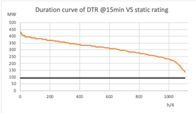
Fig. 4 Duration curve of DTR for both STR (black line) and DTR (orange line).
