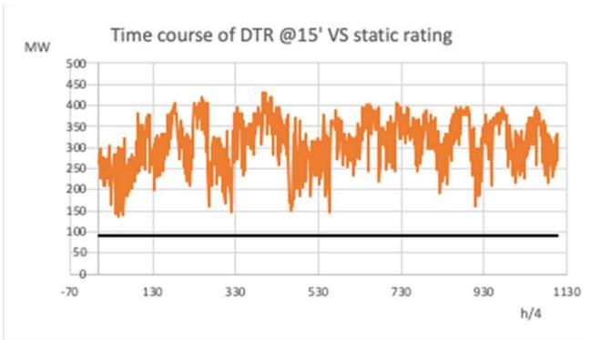
Fig. 3 Comparison between STR (black line) and DTR (orange line).
