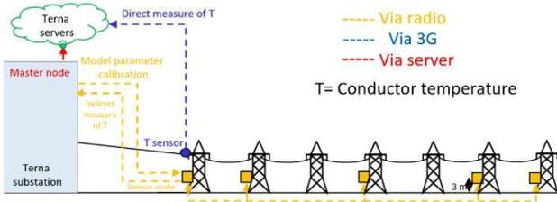
Fig. 1. Sensor-based DTR Architecture
