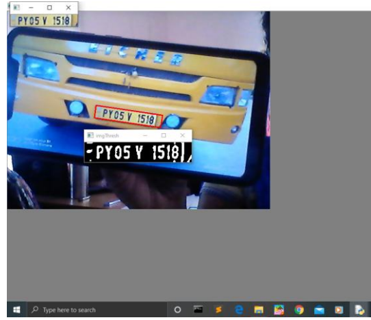
Fig 5. Experimental results for number plate detection
