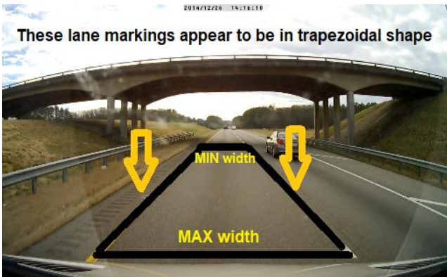
Fig. 3. The camera’s viewpoint (This figure presents the practical scenario of the road when viewed by the camera placed in the front of the car)
