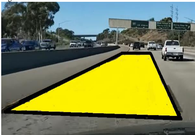
Fig. 8. Image depiction of the lane under right lane drift (This figure helps to visualize how the shape of the lane changes when the vehicle slowly starts moving to the right)
