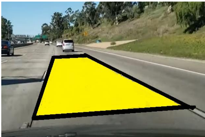
Fig. 7. Image depiction of the lane under left lane drift (This figure helps to visualize how the shape of the lane changes when the vehicle slowly starts moving to the left)
