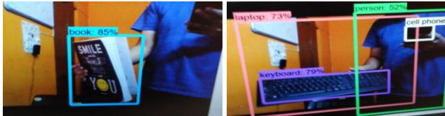
Fig. 4. Object detection using TensorFlow
