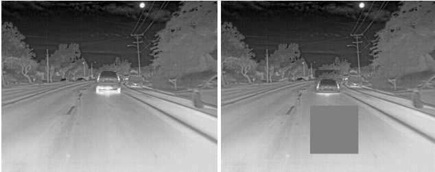
Figure 7: Left) An image from FLIR dataset; Right) BBox Augmented version. The content of the box’s car in the middle is translated downwards and a cutout square has been added.
