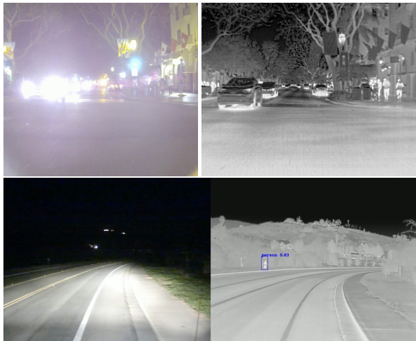
Figure 2: Top row. Left) The lights of the car headlights dazzle the RGB camera; right) cars and persons can be recognized in the same view obtained through a thermal camera. Bottom row. Left) Lack of lighting may cause dangerous situations, no pedestrian is observable in the scene. Right) the thermal camera does not depend from the intensity of the light and allows to detect the person.
