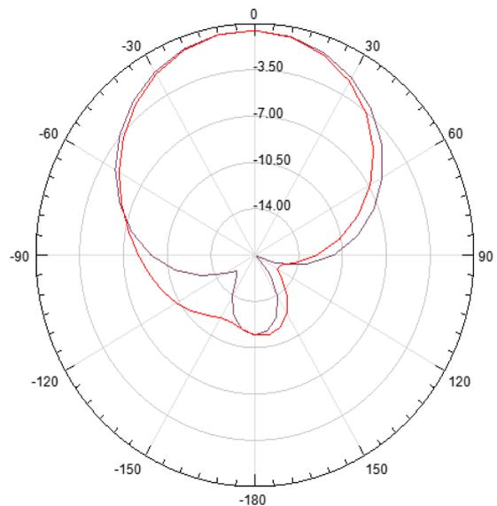
Fig.11 Proposed Reconfigurable Antenna Radiation Pattern 2.3 GHz (Both the diode D1, D2 turns ON)
