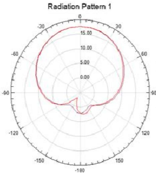
Fig.3 Conventional Antenna Radiation Pattern 2.35GHz
