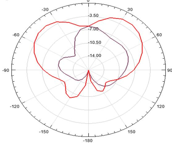
Fig.20 Proposed reconfigurable antenna Radiation pattern 4.98GHz (Diodes D1-ON and D2- OFF)
