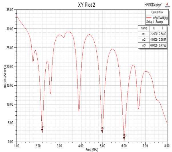
Fig.22 Proposed reconfigurable antenna VSWSR 2.2, 4.98, 6GHz (D1-ON, D2- OFF)
