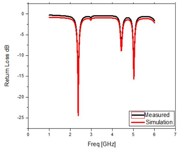
Fig.10 Proposed reconfigurable antenna return loss Simulation and Measured at 2.3,4.99GHz (Both the diode D1,D2 turns ON)
