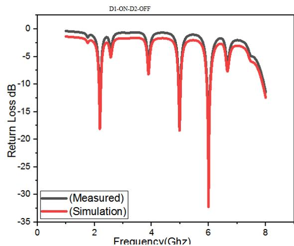
**Fig.18 Proposed reconfigurable antenna return loss Simulation and Measured at 2.2, 4.98,6 GHz (Diodes D1-ON and D2-OFF)**
