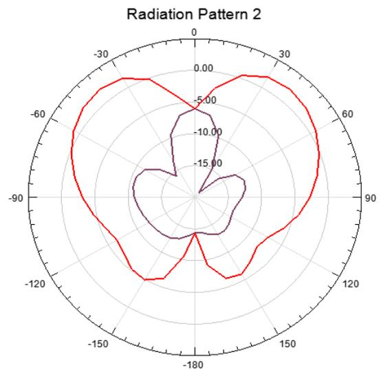
**Fig.16 Proposed reconfigurable antenna Radiation pattern 5.11GHz (Two diodes D1, D2-OFF)**
