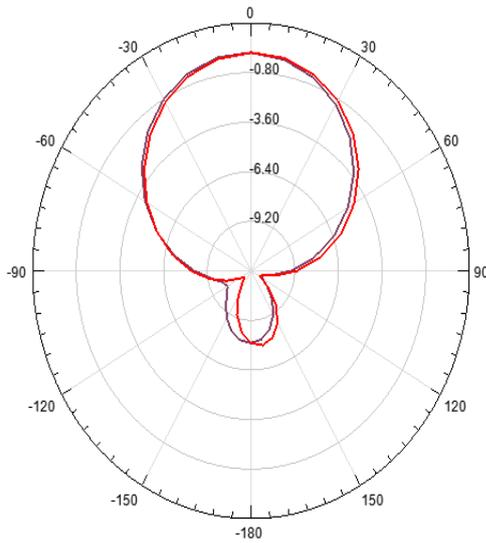
Fig.19 Proposed reconfigurable antenna Radiation pattern 2.2GHz (Diodes D1-ON and D2- OFF)
