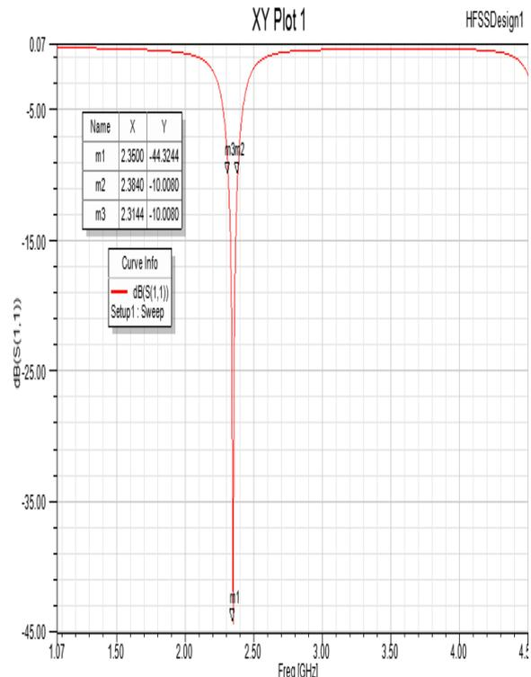
**Fig 2. Conventional Antenna Simulated Returns Loss for 2.35 GHz**
