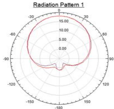
Fig.6 Modified Using U-Slot Radiation Pattern
