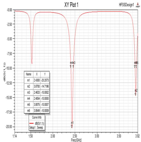
Fig.5 Modified Using U-Slot Antenna Return Loss 2.43, 3.87 GHz
