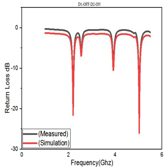
Fig.23 Proposed reconfigurable antenna return loss Simulation and Measured at 2.2,5.3 GHz (Diodes D1-OFF and D2-ON)
