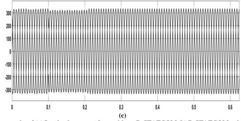
Fig.5. simulation results of (a) Load voltage waveform without D-STATCOM (b) D-STATCOM voltage waveform. (c) Load voltage waveform with D-STATCOM.
