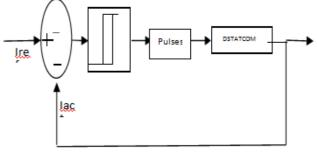
Fig.2. block diagram of hysteresis current control
