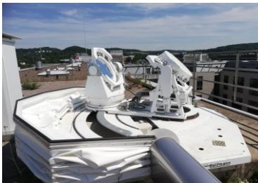
Figure 1: Siderostat of the Vacuum Vertical Telescope on the rooftop of the Institute for Astrophysics in Göttingen.
