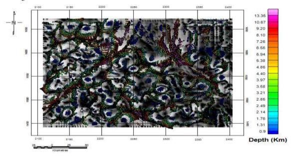
**Figure 8:-** Map of the Euler's solution for the structural indice IS=0, a window of 10x10 with a maximum relative error of about 15% on the map of the horizontal gradient of the Bouguer anomaly.
