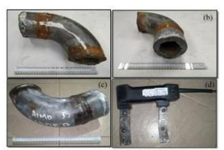
Fig 1. Failed pipe preparation for MPI
