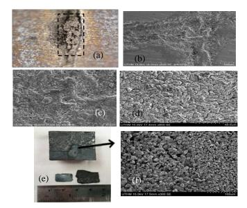
Fig 4: Crack on carbon steel at different magnification and oxide layers (right bottom).
