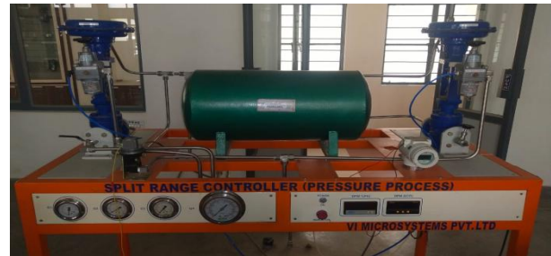
Fig.1 Pressure process station.
