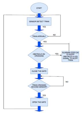
Figure 3: Flow chart showing operation of system
