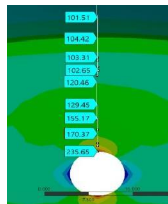
Fig. 19. Hoop stress variation along surface at 15000 RPM
