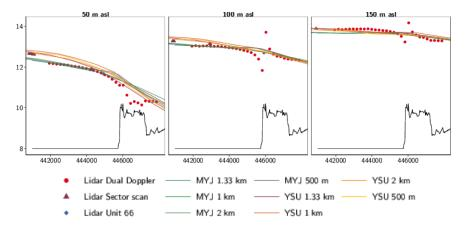
Figure: Mean wind speed using 1904 10-min measurements with 100% availability of the DD up to a distance of 5 km offshore and onshore (total 7 km - not filtered by wind direction).
