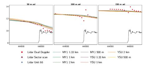
Figure: Mean wind speed using 3368 10-min measurements with 100% availability of the DD up to a distance of 2 km offshore and onshore (total 5 km).
