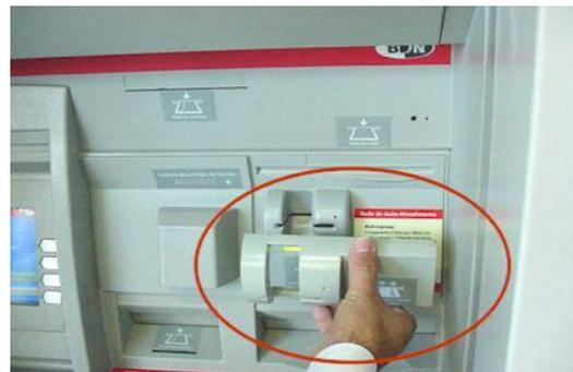
**Figure 1: Altering the slot of an ATM**
