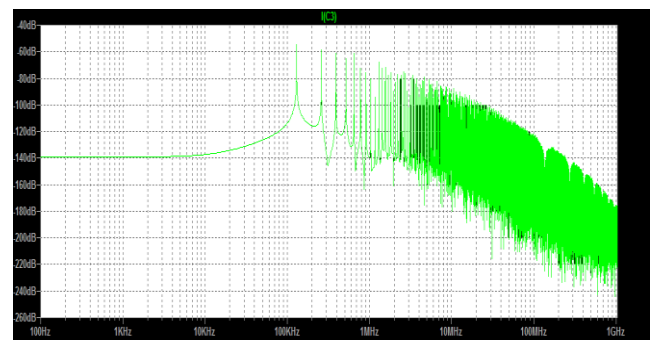
Fig 7. FFT of I_{(c3)} of Boost Equivalent Circuit (from Fig 6)
