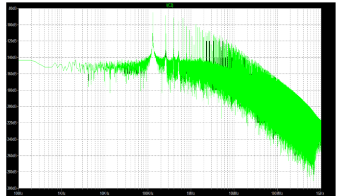
Fig 11. FFT of I (c2) of Flyback Equivalent Circuit (from Fig 10)
