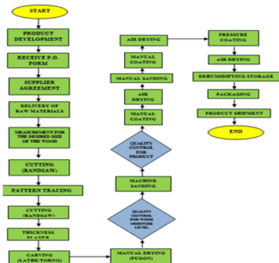
Figure 4: Company's General Process Flowchart
