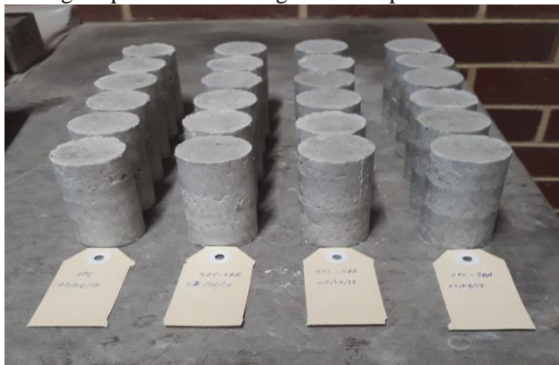
Fig. 1 Prepared UCS specimens before testing
