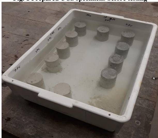
Fig 2. Specimens submerged in a magnesium sulphate basin
