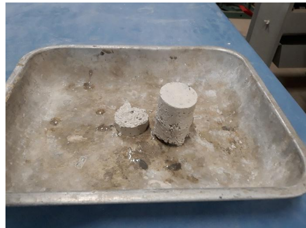
Fig. 6 Dissolved specimen after exposing to the concentration
