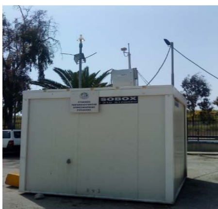
Figure 32. The Air Quality Monitoring Station in PPA SA port area.
