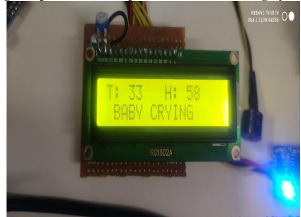
Fig.7.Measuring of temperature and humidity along with displaying whether baby crying or not
