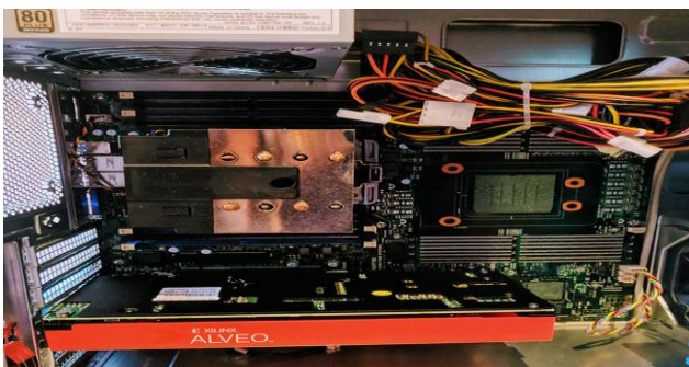
Fig .7 Alveo Board interconnected with Host
