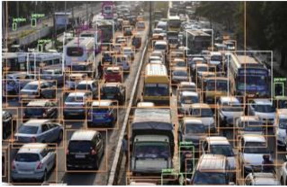
Fig. 7. Sample output for vehicle detection
