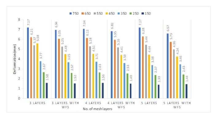
Graph 3: Deformation in (mm) For 25mm thick Ferrocement Panel
