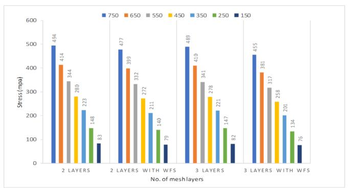
Graph 4: Equivalent Stress in (MPa) For 15mm thick Ferrocement Panel
