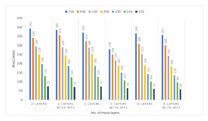
Graph 5: Equivalent Stress in (MPa) for 20mm thick Ferrocement Panel.
