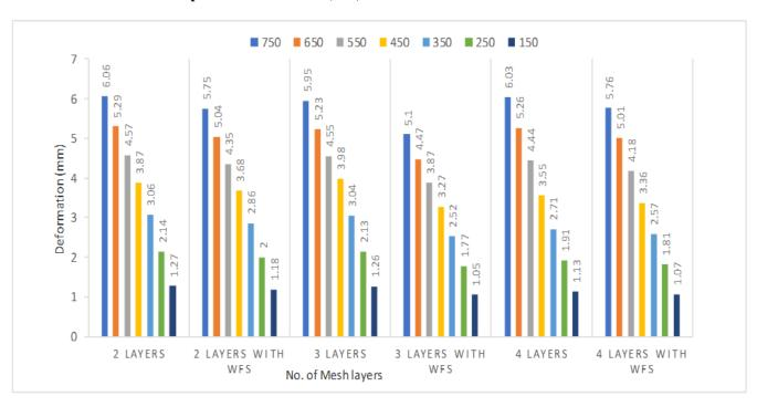
Graph 2: Deformation in (mm) For 20mm thick Ferrocement Panel
