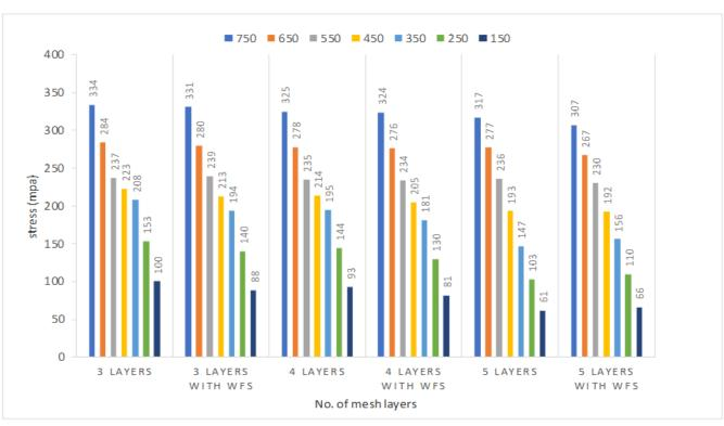
Graph 6: Equivalent Stress in (MPa) for 25mm thick Ferrocement Panel
