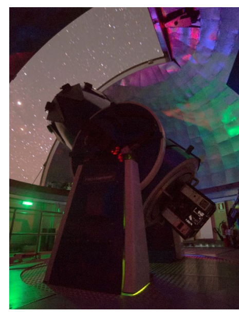
Hermes @ Mercator (ORM) Diameter = 1.2 m R ~ 85000 Range: 377 – 900 nm
