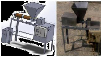
Fig 6. Hopper of the Extruder machine
