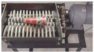
Fig 5. Plastic shredder/crusher machine
