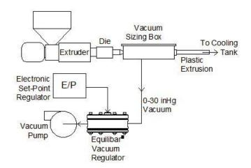
Fig 4. System Setup
