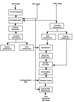
Figure 1: Flow diagram of the Proposed Fusion Scheme
